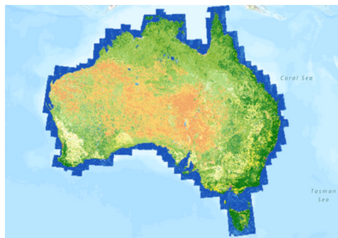
Figure 1: Map of Australia depicting land cover, observed across 30 years using Landsat imagery at a 30m resolution. Green refers to vegetation at varying densities. Source: Digital Atlas of Australia with DEA Land Cover Level 4.
